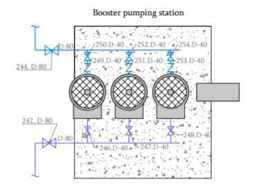
The pumping station **"Funicular I – Adjacent Settlement"** supplies the population connected to the network. The station is controlled by an automatic control panel manufactured by **Grundfos**, which maintains constant pressure in the discharge network. The control process is fully automated.
