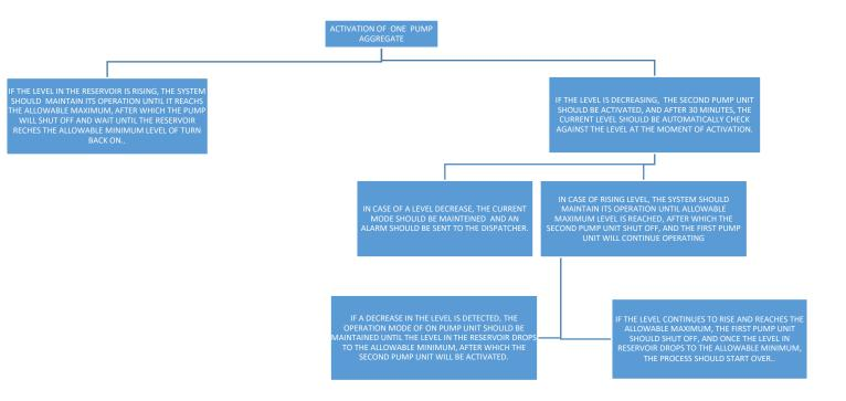
In summer mode, due to the relatively higher demand for flow, the pumping station operates in a variable mode, based on the 1-2 principle. In this mode, the simultaneous operation of two pumps is required to fill the reservoirs. After filling is completed, one pump remains in operation. If the maximum emergency level is reached, the remaining pump unit is also shut down.
