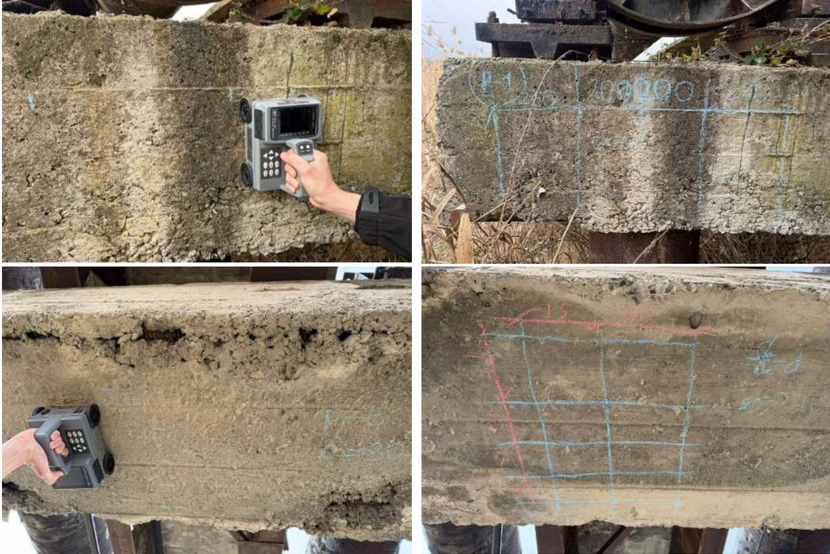
*Fig. 15. Determination of the reinforcement location and the protective layer of concrete using "NJJ-105 Hand Search"*
