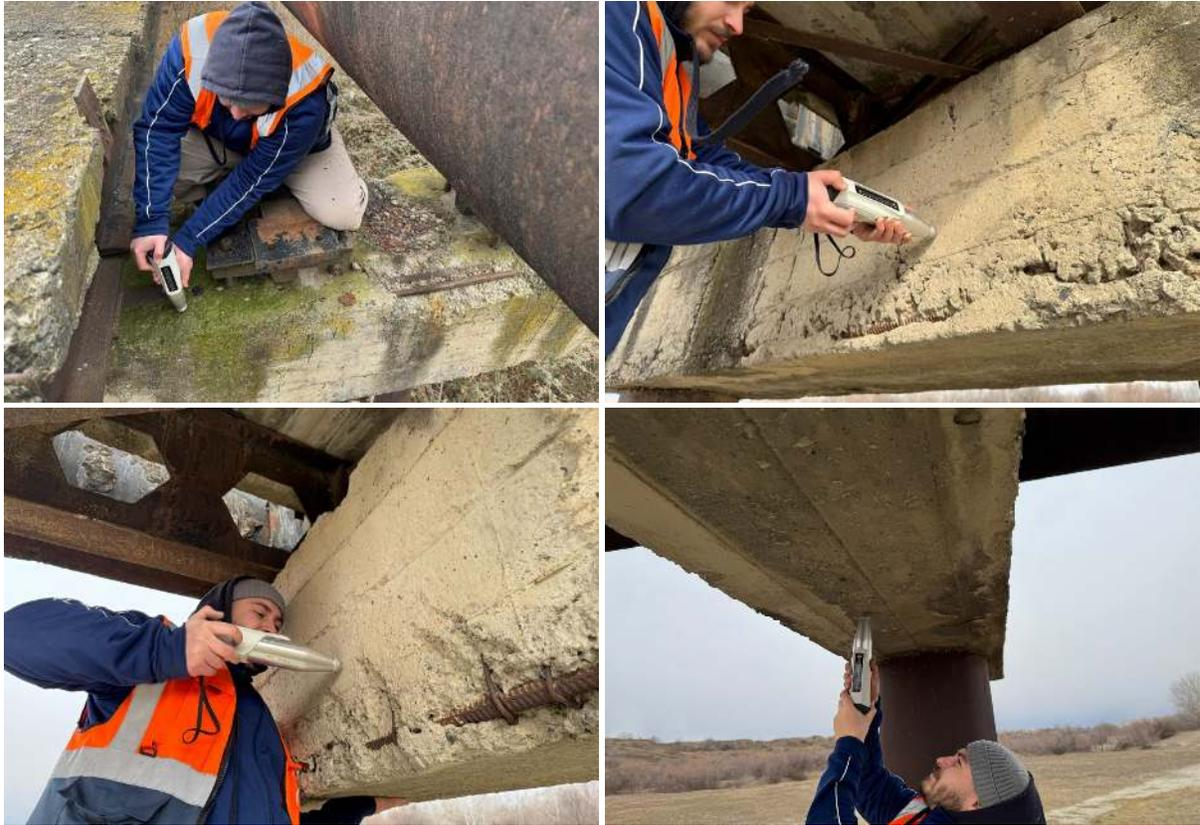
*Fig. 14. Determination of the concrete class by Silver Schmidt.*
