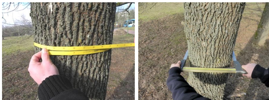
Measuring DBH with a tape (left) and a diameter calliper (right).
